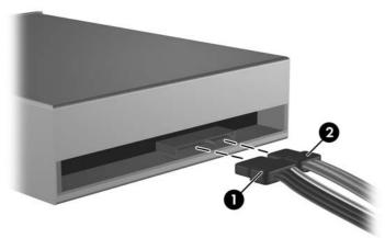
7. Remove the screw that secures the drive to the drive cage (1), then slide the drive out of the front of the chassis (2).
